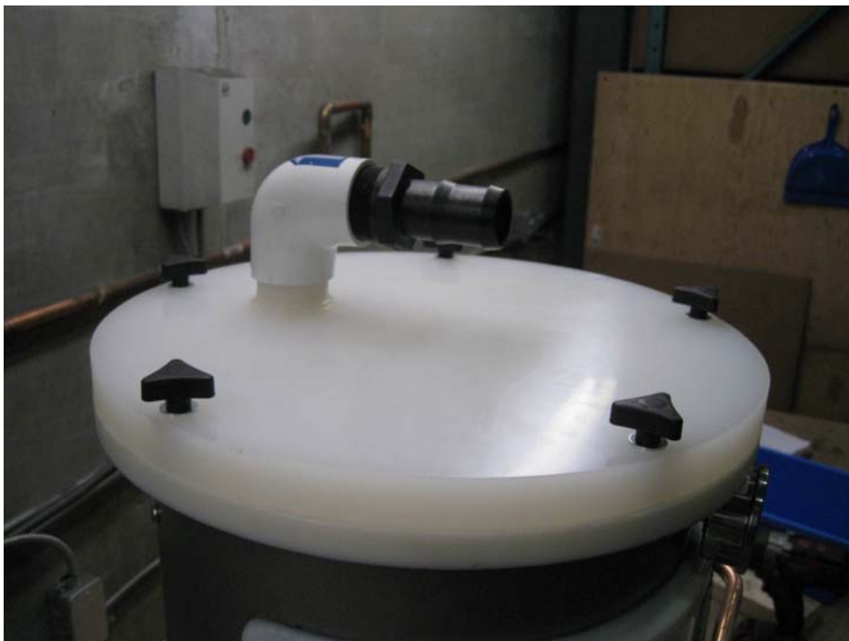
Connect hose from Dental inlet to hose barb connector
